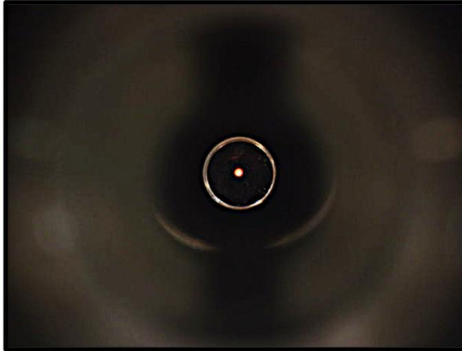
**Figure 5.7:** Photograph of the realigned collector looking down the axis of the beam line. The cathode is warm and glowing in the centre of the photograph. The collector assembly, illuminated by the cathode, and is on-axis with both the electron gun and the beam line.
