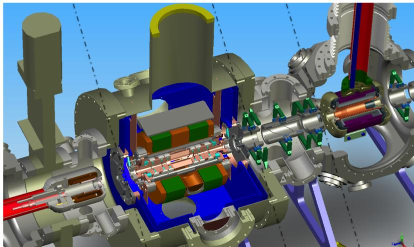
**Figure 2.8:** Schematic of the TITAN EBIT. From left to right: the electron gun assembly, the magnet chamber and drift tube assembly, the injection optics, and the collector assembly (Credit: Image Courtesy of TITAN).
