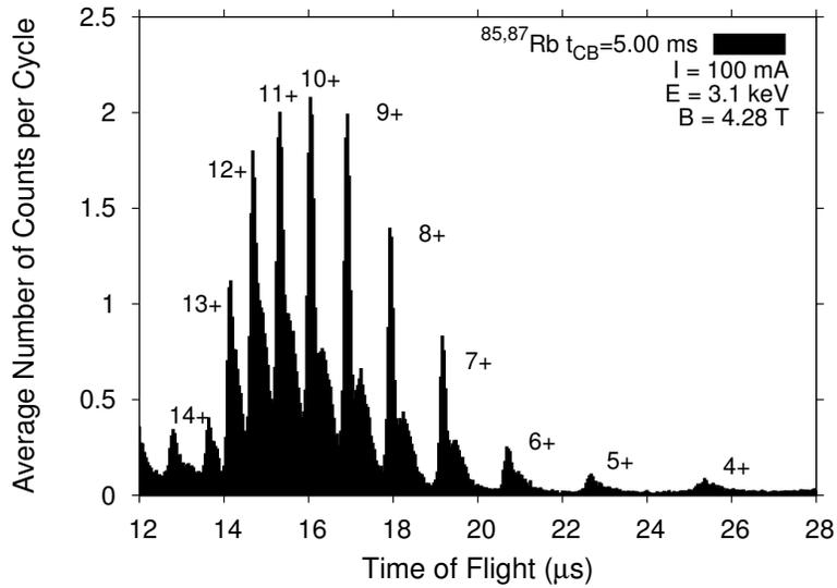
**Figure 5.1:** Time-of-flight spectrum of charge-bred Rb for  $E = 3.1$  keV,  $I = 100$  mA,  $B = 4.28$  T, and  $t_{CB} = 5$  ms. Higher charge states appear at a longer time of flight. The charge states of Rb 4+ to 14+ are labeled.
