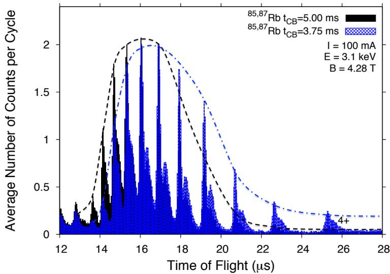
**Figure 5.2:** Time-of-flight spectra of charge-bred  $^{85,87}\text{Rb}$  for  $E = 3.1$  keV,  $I = 100$  mA,  $B = 4.28$  T, and  $t_{CB} = 3.75$  ms (shaded blue) and 5 ms (solid black). An envelope passes through the peak number of counts in each charge state to show qualitative differences between the two distributions (details in text). No corrections have been made for background or residual gas ions.
