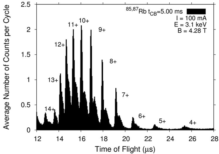
**Figure 5.8:** Time-of-flight spectrum of charge-bred  $^{85,87}\text{Rb}$  for  $E = 3.1$  keV,  $I = 100$  mA,  $B = 4.28$  T, and  $t_{CB} = 5$  ms for comparison to CBSIM. The charge-state distribution peaks at  $q = 10+$  with a small but non-negligible amounts in the 5+ and 15+ charge states.
