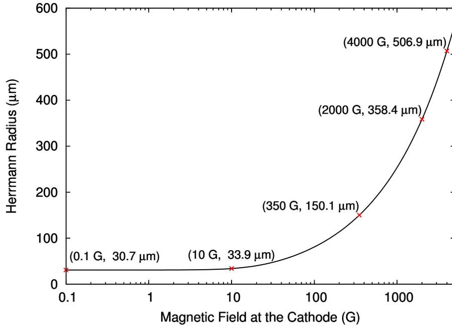
**Figure 2.10:** Herrmann radius of the electron beam as a function of the residual magnetic field at the cathode for typical values in the TITAN EBIT:  $T_c = 1470$  K,  $r_c = 0.00170$  mm,  $B = 4.5$  T,  $E = 2.5$  keV,  $I_e = 0.100$  mA.
