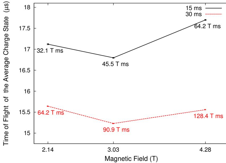
**Figure 5.5:** Results of changing the magnetic field strength in the trapping region and charge-breeding time on the production of charge-state distributions. The  $\bar{T}(\delta T)$  from each charge-state distribution is plotted against the value of  $B$  for different charge-breeding settings. Lines connect constant charge-breeding time (15 ms in solid black, 30 ms in dashed red) and labels indicate the product of  $B$  and  $t_{CB}$ .
