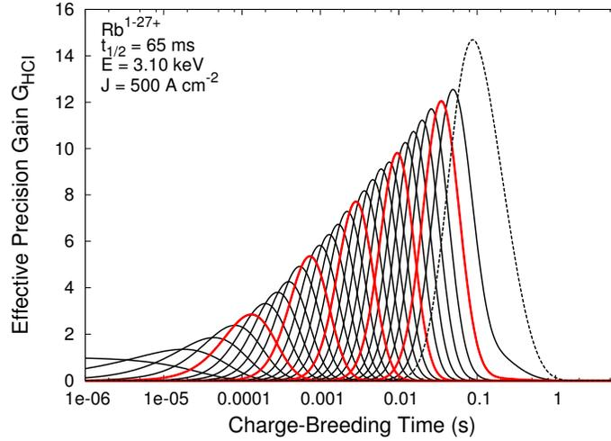
**Figure 4.5:** Evolution of  $G_{HCI}(q, t_{CB}, 500 \text{ A cm}^{-2}, 3.1 \text{ keV})$  for  $^{74}\text{Rb}^{q+}$  ( $t_{1/2} = 65 \text{ ms}$ ). The maximum precision gain occurs in the 27+ charge state since the increased current density makes threshold effects advantageous before radioactive decay-losses diminish  $G_{HCI}$ . Every fifth charge state (bold red) and the maximum charge state (dashed black) are emphasized to guide the eye.
