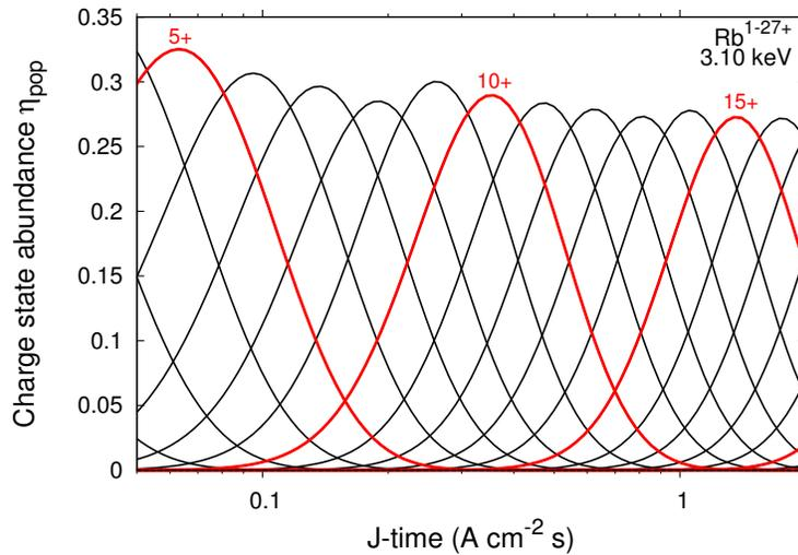
**Figure 5.9:** Charge-state evolution of  $^{85}\text{Rb}^{7+}$  for threshold charge-breeding conditions at  $E = 3.1$  keV for comparison to an experimental charge-state distribution. The 10+ charge state peaks for a J-time  $\approx 0.35$  A  $\text{cm}^{-2}$  s and there is a near-negligible fraction of ions in the 5+ and 15+ charge states (red) at this value of J-time.
