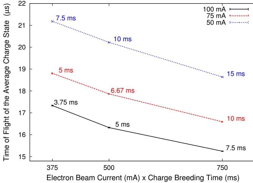
**Figure 5.4:** Results of changing the electron-beam current and charge-breeding time on the production of charge-state distributions. The  $\bar{T}(\delta T)$  from each charge-state distribution is plotted against the product of  $I$  and  $t_{CB}$  for the different charge-breeding settings. Lines represent constant electron-beam current (100 mA in solid black, 75 mA in dashed red, 50 mA in dotted blue) and labels indicate the  $t_{CB}$ .
