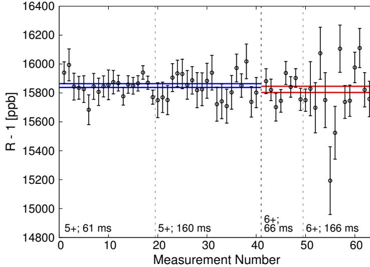
**Figure 6.4:** Cyclotron frequency ratios between  $^{51}\text{V}^{q+}$  and  $^{51}\text{Cr}^{q+}$  for different excitation times and charge states. Each point represents the ratio resulting from a single  $^{51}\text{Cr}^{q+}$  resonance and its neighbouring  $^{51}\text{V}^{q+}$  resonances. The blue (left) and red (right) lines show the  $1\sigma$  error band for all 5+ and 6+ ratio measurements, respectively.
