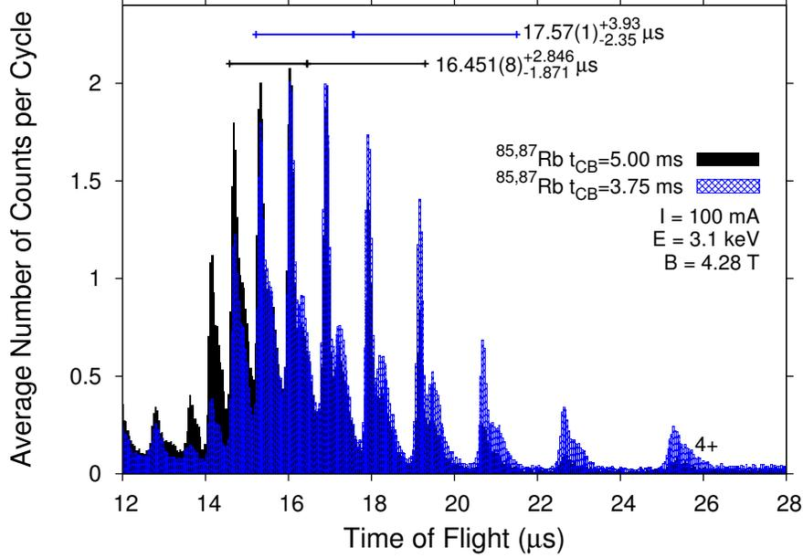
**Figure 5.3:** Time-of-flight spectra of charge-bred  $^{85,87}\text{Rb}$  for  $E = 3.1$  keV,  $I = 100$  mA,  $B = 4.28$  T, and  $t_{CB} = 3.75$  ms (shaded blue) and 5 ms (solid black). The time of flight of the average charge state and the asymmetric widths are shown at the top of the graph in the format  $\bar{T}(\delta T) \sigma_{-}^{+}$ .
