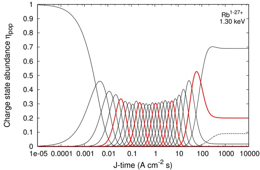
**Figure 4.1:** Charge-state evolution of  $\text{Rb}^{q+}$  for  $E = 1.30$  keV. A vertical slice at fixed time shows the charge-state distribution of an ion bunch after a given J-time. Every fifth charge state (bold red) and the maximum charge state (dashed black) are emphasized to guide the eye.
