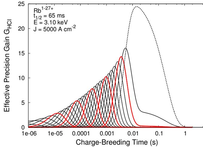
**Figure 4.6:** Evolution of  $G_{HCI}(q, t_{CB}, 5000 \text{ A cm}^{-2}, 3.1 \text{ keV})$  for  $^{74}\text{Rb}^{q+}$  ( $t_{1/2} = 65 \text{ ms}$ ). The maximum precision gain occurs in the 27+ charge state and the full advantage of the threshold effect is available resulting in  $G_{HCI} \approx q$ . Every fifth charge state (bold red) and the maximum charge state (dashed black) are emphasized to guide the eye.
