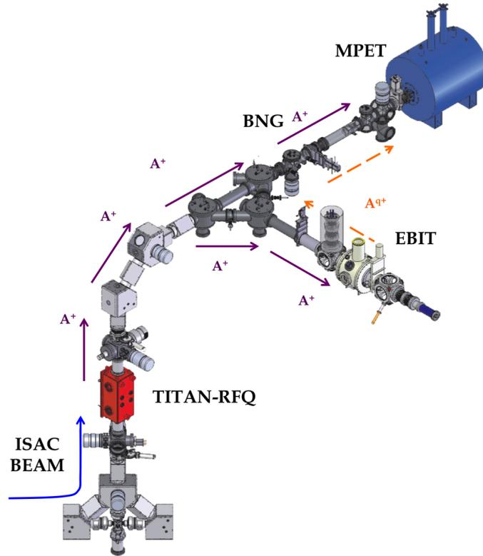
**Figure 3.2:** The TITAN experiment depicting the location of the TITAN RFQ, the EBIT, the Bradbury-Nielsen gate (BNG), and the MPET. The respective ion paths are shown for SCI  $A^+$  (solid purple) and for HCI  $A^{q+}$  (dashed orange) (Credit: Image Courtesy of TITAN).
