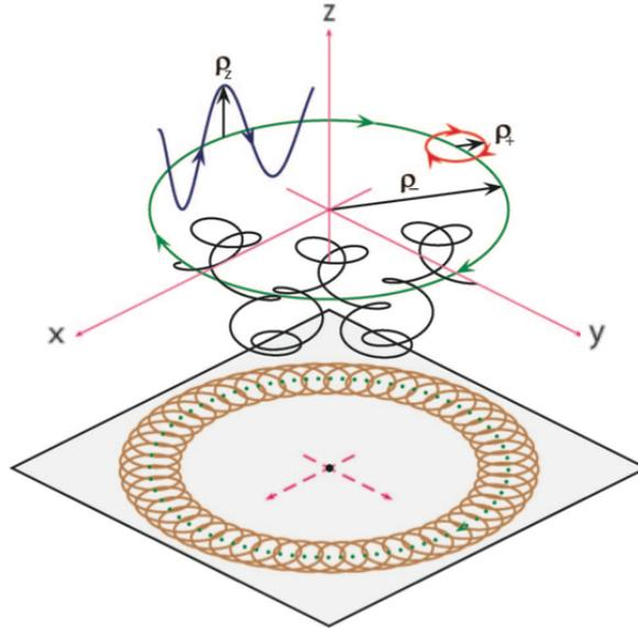
**Figure 2.4:** Trajectory of an ion in a Penning trap. The combined motion (black) and independent eigenmotions are shown: harmonic oscillation in the axial direction (blue); reduced cyclotron motion (green) and magnetron motion (red) (figure from Ref. [29] ©2010 Taylor & Francis. Reproduced with permission).
