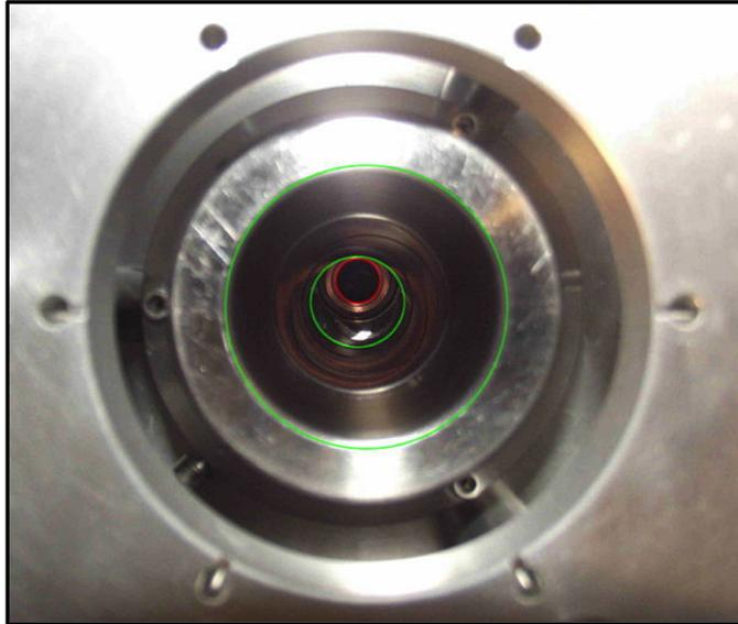
**Figure 5.6:** Photograph of the collector misalignment looking down the axis of the beam line. The front and back ends of the ion injection optics (green) and the front of the collector assembly (red) are visible. The collector assembly is 7 mm off of the beam line axis.
