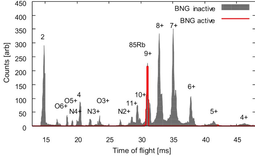
**Figure 3.4:** Time-of-flight spectra of highly charged ions after being extracted from the EBIT with and without Bradbury-Nielsen gate (BNG) operation.  $^{85}\text{Rb}$  charge states 4-11+ are marked, as are peaks of nitrogen, oxygen, and other gas ions ( $\text{O}^{q+}$ ,  $\text{N}^{q+}$ ). The red spectrum identifies the  $^{85}\text{Rb}^{9+}$  that has been selected by the BNG for injection into the MPET (details in text).
