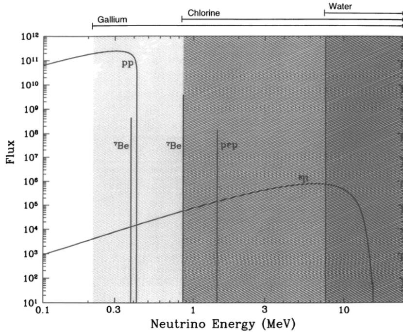
**Figure 6.1:** Energy spectrum of solar neutrinos and energy thresholds for neutrino detectors. The energy spectrum of the neutrinos from the p-p chain as predicted by the Standard Model is shown. The arrows at the top indicate the energy sensitivity of different neutrino detectors (figure from [91] ©AAS. Reproduced with permission).
