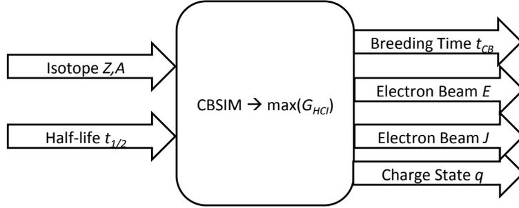
**Figure 4.11:** Schematic outline of the optimization procedure for  $G_{HCl}$ . By specifying the isotope of interest and its half-life, the optimization provides the optimal  $q$ ,  $t_{CB}$ ,  $E$ , and  $J$ , fully specifying the optimal charge-breeding conditions for PTMS with highly charged, radioactive ions.
