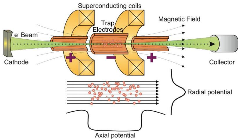
**Figure 2.7:** Illustration of an EBIT. From left to right: the electron gun assembly, the magnet coils and drift tube assembly, and the collector assembly. Typical trapping potentials are shown. (figure from Ref. [38] ©Maxime Brodeur. Reproduced with permission).
