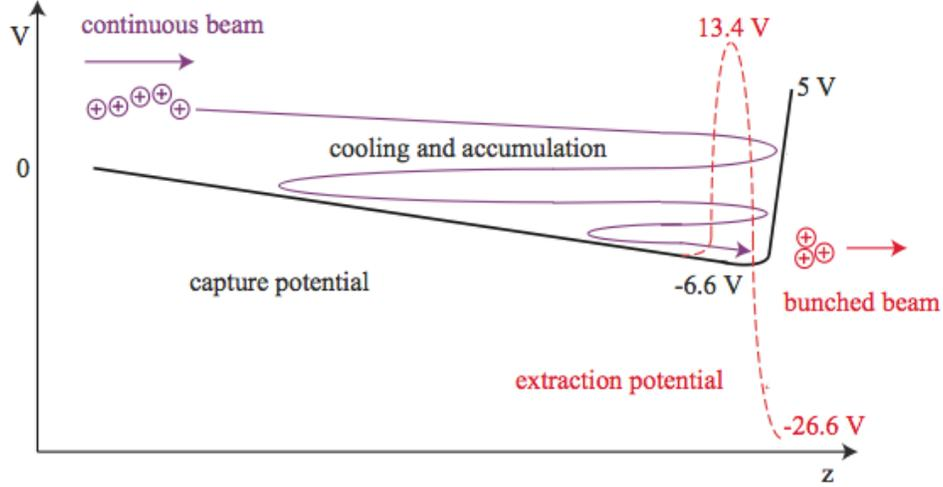
**Figure 2.3:** Schematic of the axial trapping (black) and extraction (red) potentials for the TITAN RFQ. The extraction potential is used to create an ion bunch separate from the incoming continuous beam (purple) (figure from Ref. [38] ©Maxime Brodeur. Reproduced with Permission).
