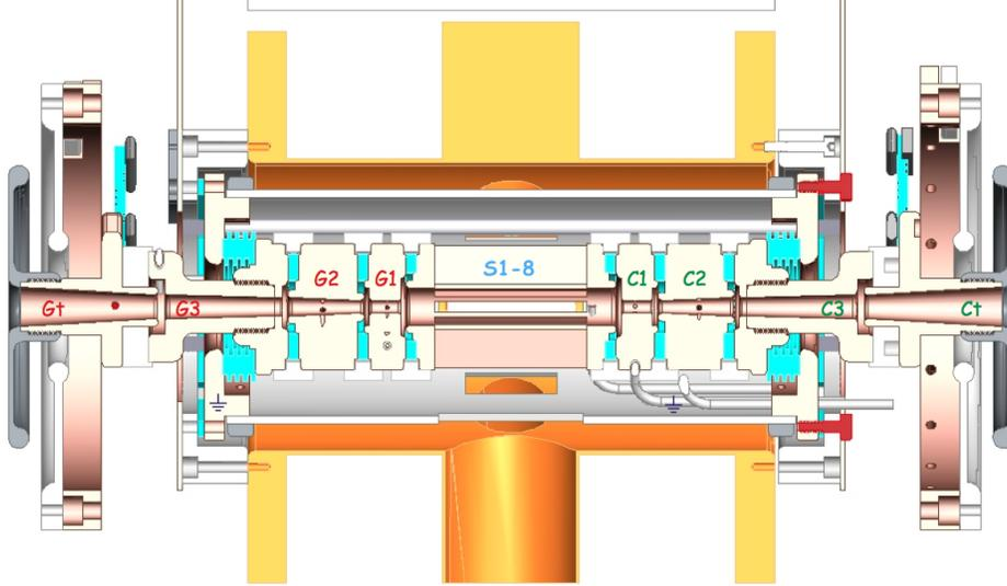
**Figure 3.3:** The trapping region of the TITAN EBIT. The trap drift tubes are labeled out from the central drift tube (S) towards either the gun (G) or collector (C) assembly, with C1 corresponding to the first drift tube on the collector side and so on. S1 through S8 denotes the eight segments of the central drift tube (Credit: Image Courtesy of TITAN).
