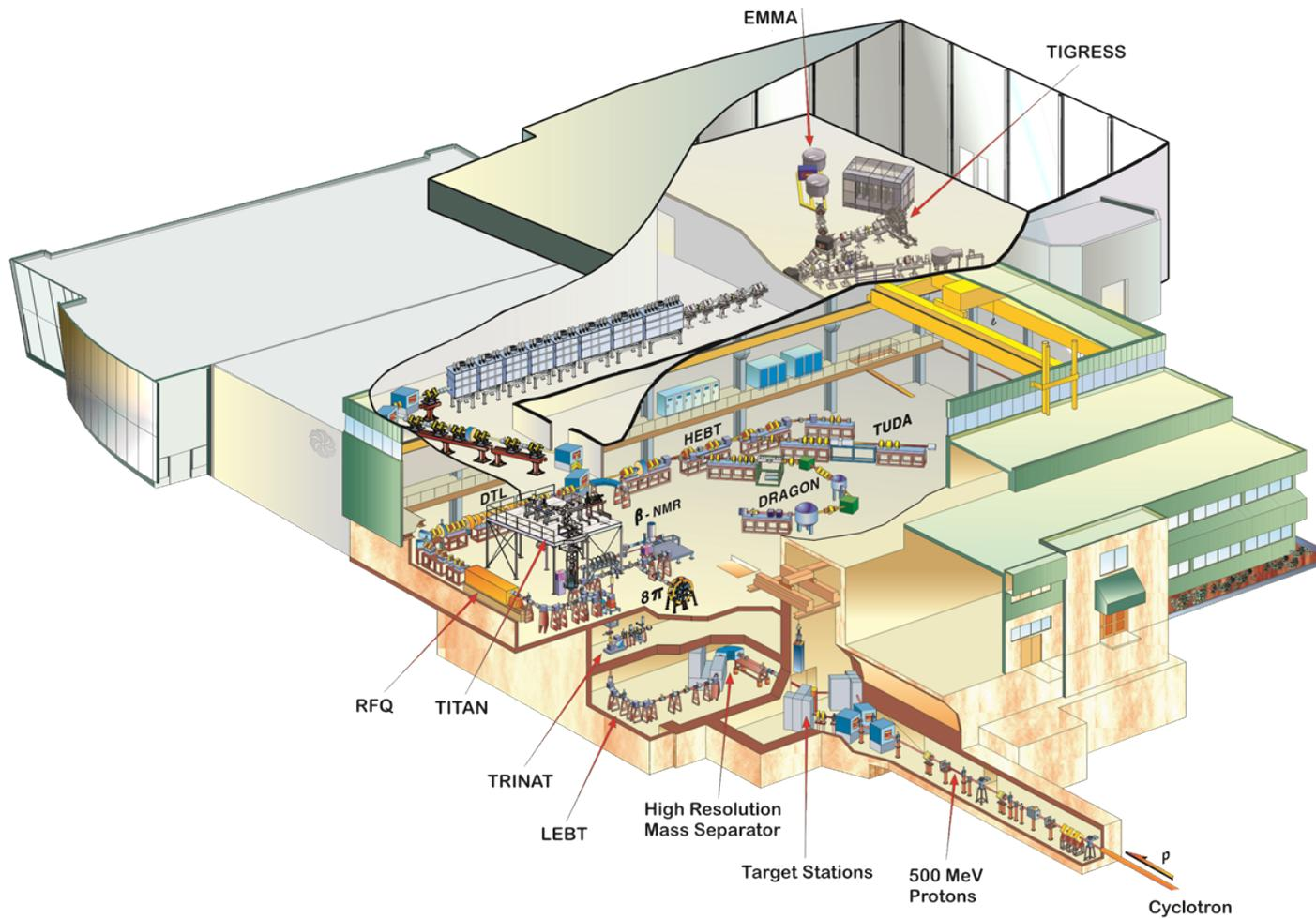
**Figure 3.1:** The experimental halls at ISAC. The beam line for the ISOL production of radioactive ions at TRIUMF is shown, and includes the proton beam line, target / ion source combination, mass separator, and ion transport system. Various experimental setups, including TITAN, are shown. (Credit: Image Courtesy of TRIUMF).
