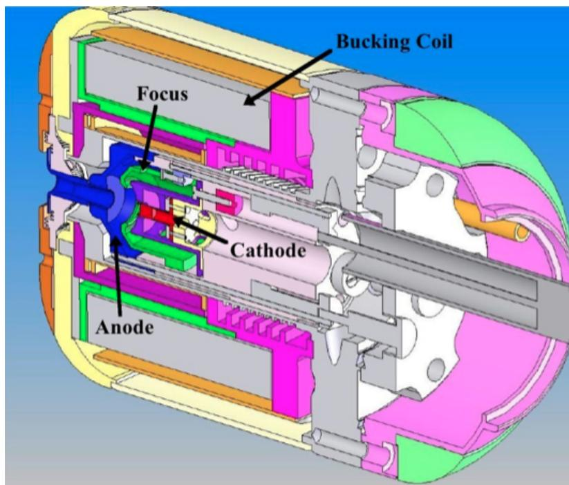
**Figure 2.9:** Cross-section view of the EBIT gun assembly at TITAN. The cathode (red) emits the electrons, which are pulled by the focus (dark green) and accelerated towards the left through the anode (blue). The bucking coils (grey) are used to reduce the residual magnetic field at the cathode (Credit: Image Courtesy of TITAN).
