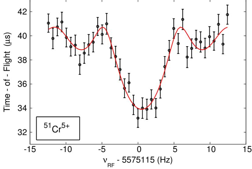
**Figure 6.3:** A TOF-ICR resonance for  $^{51}\text{Cr}^{5+}$  with a  $T_{RF} = 160$  ms excitation. The solid line is a fit of the theoretical line shape [42] to the data.
