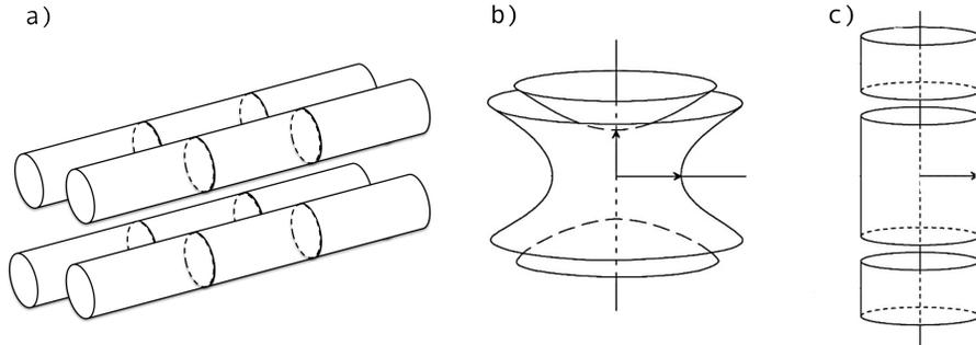
**Figure 2.1:** Typical ion trap electrode configurations: a) linear trap consisting of four segmented rods; b) hyperbolic trap consisting of two end caps and a ring electrode; and c) cylindrical trap consisting of a series of cylindrical electrodes (drift tubes) (modified figures b) and c) from Ref. [29] ©2010 Taylor & Francis. Reproduced with permission).
