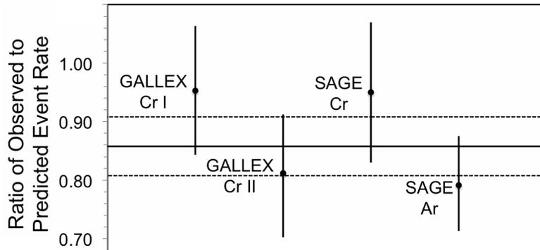
**Figure 6.2:** Ratio of observed to predicted event rate for the neutrino source experiments at SAGE and GALLEX. The results of the two  $^{51}\text{Cr}$  experiments at GALLEX and both the  $^{51}\text{Cr}$  and  $^{37}\text{Ar}$  experiments from SAGE are shown. The the weighted average (solid) and the its uncertainty (dashed) of the four results (data from Ref. [27]).
