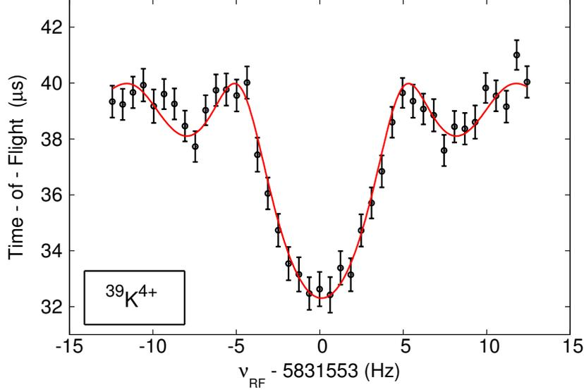
**Figure 2.6:** A TOF-ICR resonance curve for  $^{39}\text{K}^{4+}$  with a  $T_{RF} = 166$  ms excitation. The average time-of-flight and one standard deviation uncertainties (black) are shown with a theoretical fit [42] to the data (red) as a function of the excitation frequency  $\nu_{RF}$ .
