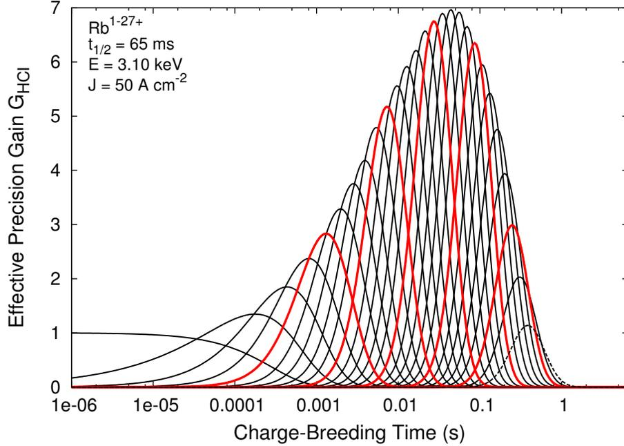
**Figure 4.4:** Evolution of  $G_{HCI}(q, t_{CB}, 50 \text{ A cm}^{-2}, 3.1 \text{ keV})$  for  $^{74}\text{Rb}^{q+}$  ( $t_{1/2} = 65 \text{ ms}$ ). The maximum precision gain occurs in the 17+ charge state for  $t_{CB} \approx t_{1/2}$ . When the charge-breeding time exceeds the half-life,  $G_{HCI}$  falls off due to losses from radioactive decay. Every fifth charge state (bold red) and the maximum charge state (dashed black) are emphasized to guide the eye.
