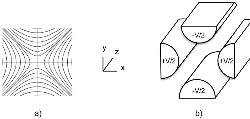
**Figure 2.2:** Radial cross-section of a linear Paul trap: a) equipotential lines of the quadrupole field, and b) electrode configuration. Neighbouring electrodes are of opposite polarity to generate the quadrupole field, which is switched at a radio-frequency to provide radial ion confinement.
