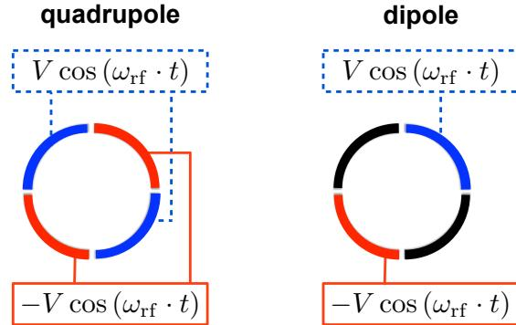
**Figure 3.31:** Schematic of a cross sectional view of a segmented ring electrode which can be used to apply an azimuthal quadrupole or dipole field on top of the DC trapping potential.
