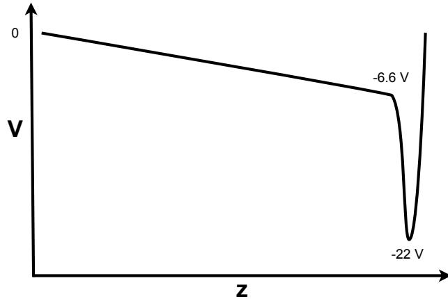
**Figure 3.11:** Schematic of RFQ DC potential during the neutron deficient Rb-mass measurements.
