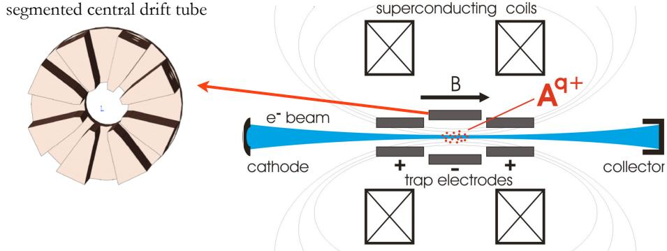
**Figure 3.13:** Right: Schematic of an EBIT with a magnetic field formed by Helmholtz coils. The ions are trapped in axial direction by an electrostatic field. Left: A cross sectional view of the central trapping electrode. It is segmented which provides direct visual access to the trapped HCl and allows monitoring of the charge breeding process. Moreover, the segmentation can be used for RF- cleaning (see Section 3.7.6).
