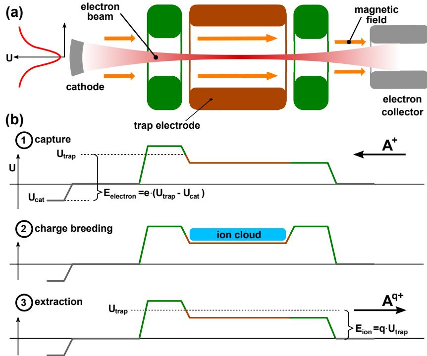
**Figure 3.15:** Schematic of the EBIT (a) and the injection, charge breeding, and extraction potentials (b).
