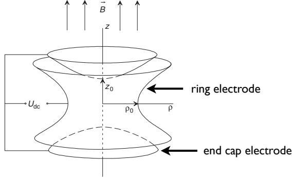
**Figure 3.22:** Schematics of a Penning trap. The hyperbolic shape of the electrodes generates the electrostatic quadrupole potential of Equation 3.4. Figure modified from [5].
