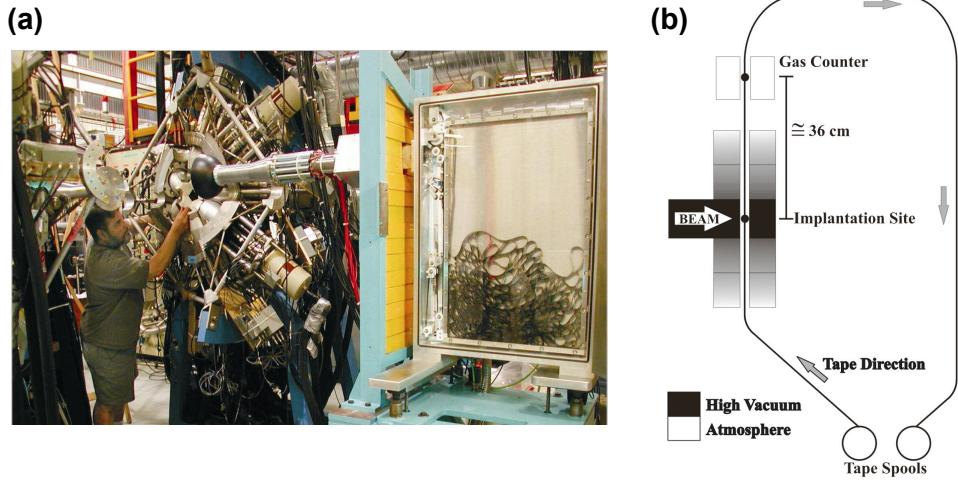
**Figure 3.5:** (a) Photo of the  $8\pi$  facility. (b) Schematic of the gas proportional counter with tape station. Both from [153].
