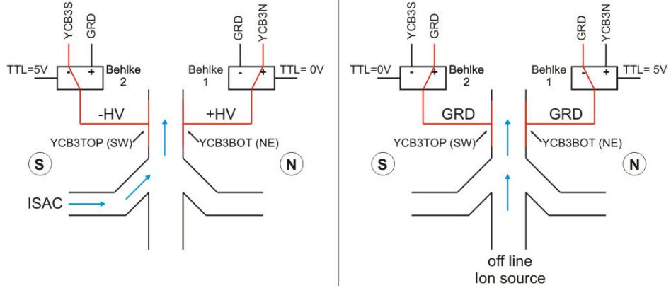
**Figure A.4:** Schematic of the beam gate in front of the RFQ for controlled injection times of ions from either ISAC or TITAN’s ion source. Either the ISAC beam or the ion source is blocked completely by a source cup or a gate valve. By switching the bias voltage of steerer plates YCB3TOP and YCB3BOT, the steerer plates act as a beam gate. In the configuration pictured on the left the ISAC is injected into RFQ, while for the case on the right only a beam sent from TITAN’s ion source can pass.
