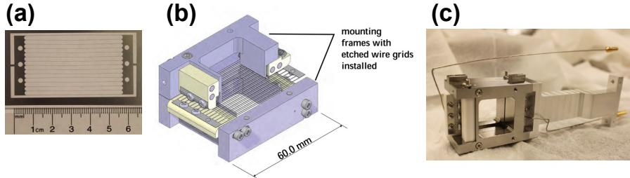
**Figure 3.21:** New design of BNG based on chemically etched wires. The etched wires (a), the schematic of the BNG (b), and the fully assembled BNG (c) are shown. Figures from [174].
