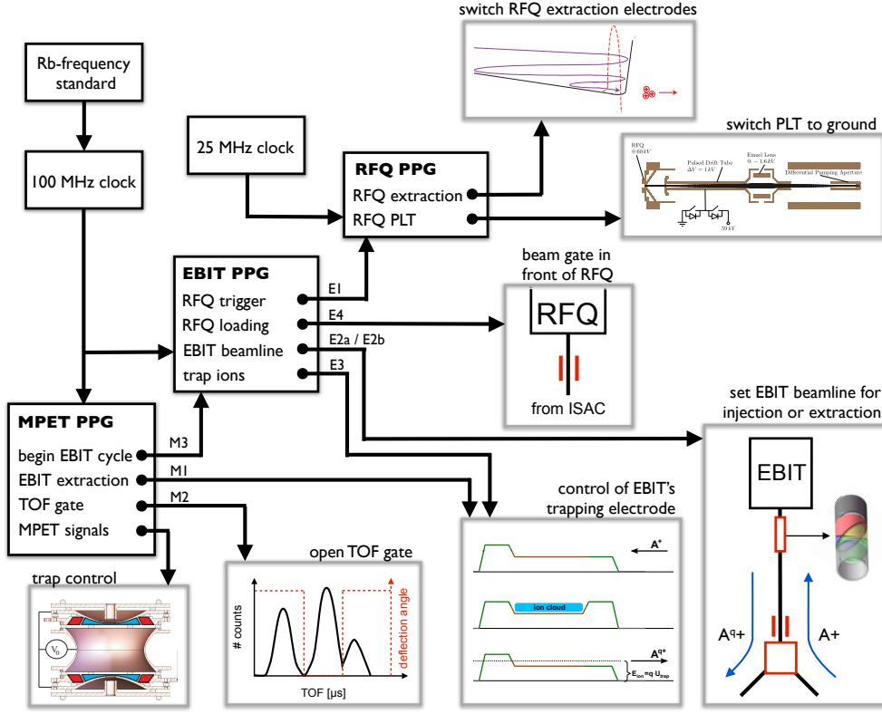
**Figure A.6:** Hierarchy of experimental control with Programmable Pulse Generators (PPGs).
