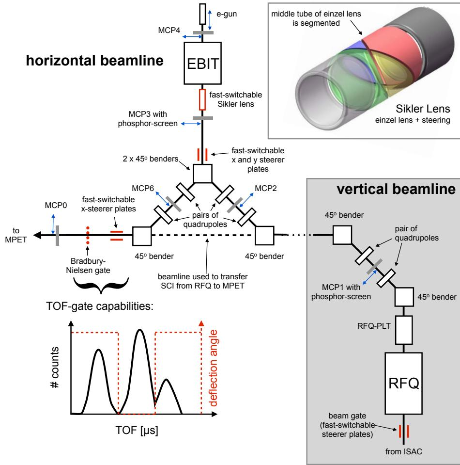
**Figure 3.19:** Layout of the TITAN transport beamline from the RFQ cooler and buncher to the EBIT and finally to the MPET. Only the elements which are mentioned in the text are displayed while omitting other einzel lenses and steerers. Elements displayed in red are controlled by fast HV switches. Devices with blue double arrows are retractable. The insert at the top right shows a schematic of a so-called Sikler lens. Figure of the Sikler lens taken from [172].
