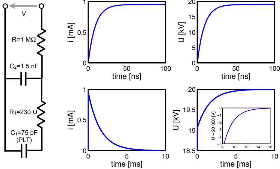
**Figure A.2:** Circuit diagram representing the switching from ground potential to 20 kV (on the left) (+HV branch in Figure A.1). The graphs on the right show the current drawn from the power supply and the voltage at the PLT. While the plots in the first row show changes in the first 100 ns, the row of plots at the bottom illustrate the long term (10 ms) behaviour.
