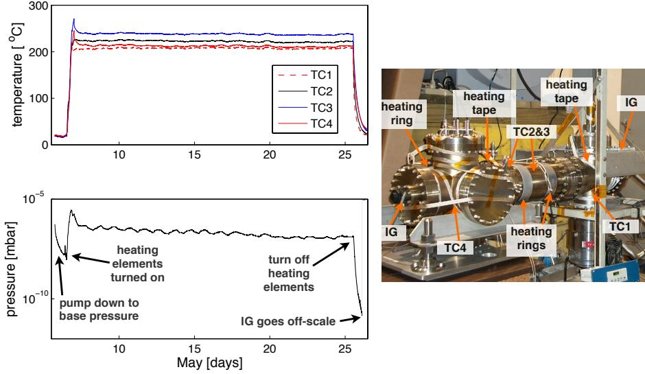
**Figure A.10:** Baking of the detector cross and the new beam optics elements along the extended extraction path. The picture on the right shows all heating and diagnostics devices before being wrapped in Al-foil and insulating material. The graphs on the left display temperatures and pressure during the baking.
