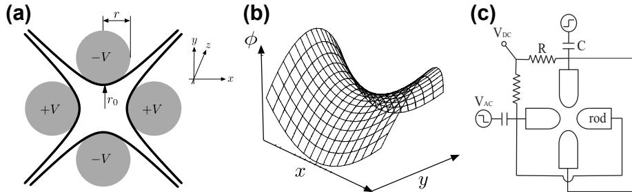
**Figure 3.9:** Schematic cross sectional view of electrode structure (a), which generates a radial quadrupole field (b). The polarity of the applied potentials in (a) is switched following a square-wave RF driver, which confines the ions radially. The coupling of the DC and RF components to the individual electrodes of a longitudinal segment is shown in (c). Figure (a) and (b) are from [134] and (c) from [146].
