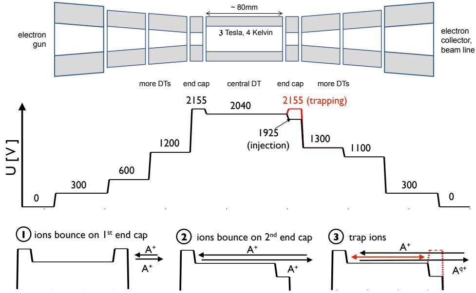
**Figure A.5:** Schematic of the EBIT drift tubes (top) and their potentials (bottom) for injection and trapping during the charge breeding of neutron-deficient Rb- isotopes. The procedure for the optimization of the ion injection is shown in (1) to (3). Electrode structure modified from [235].
