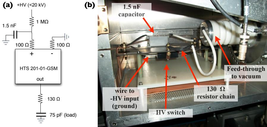
**Figure A.1:** HV switch setup to bring the PLT from maximal 20 keV to ground potential.(a) is the a circuit diagram and (b) a photo of the setup.
