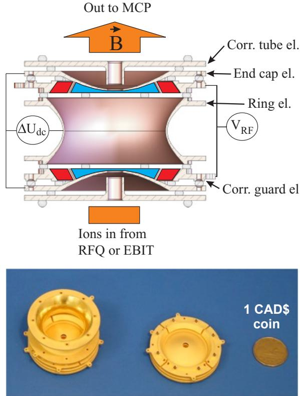
**Figure 3.33:** Schematics and picture of TITAN’s MPET electrodes. The Canadian dollar coin (with a diameter of 26.5 mm) is given for scale (bottom). Figures from [146].
