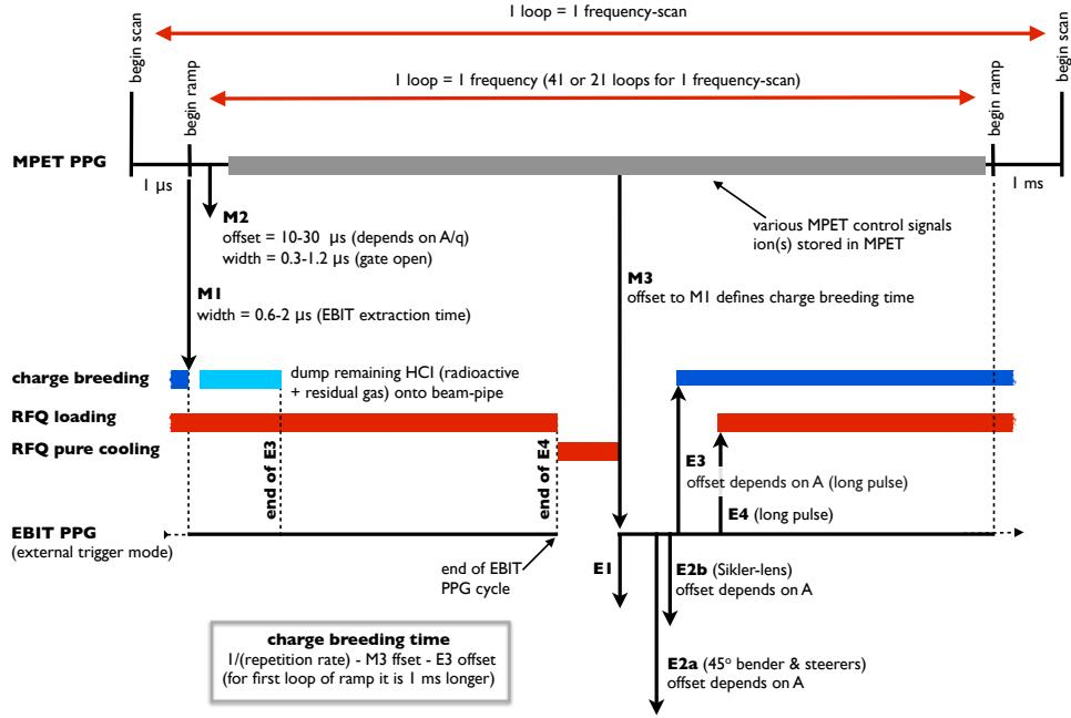
**Figure A.7:** Schematic of timings of MPET and EBIT PPG for beam transport and charge breeding. The signal names (e.g. M2) refer to the names given in Figure A.6. Timings on the x-axis are not to scale.
