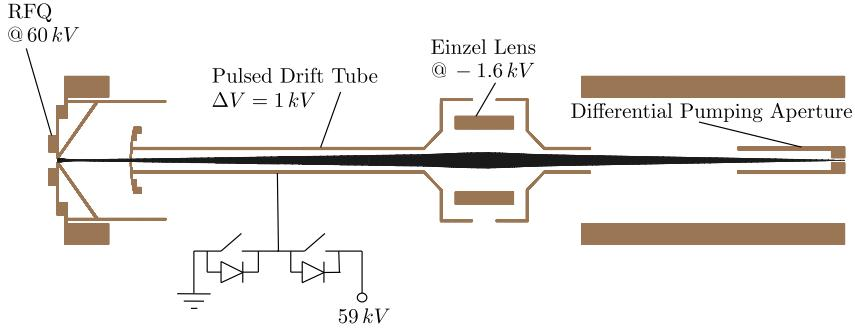
**Figure 3.12:** Extraction optics from the RFQ into a PLT which is floated to  $U_{\text{RFQ}} - \Delta V$ . When the ion bunch is in the centre of the PLT it is switched to ground without affecting the ion bunch. The SCI leave the PLT with a kinetic energy of  $e \cdot \Delta V$ . Figure from [134].
