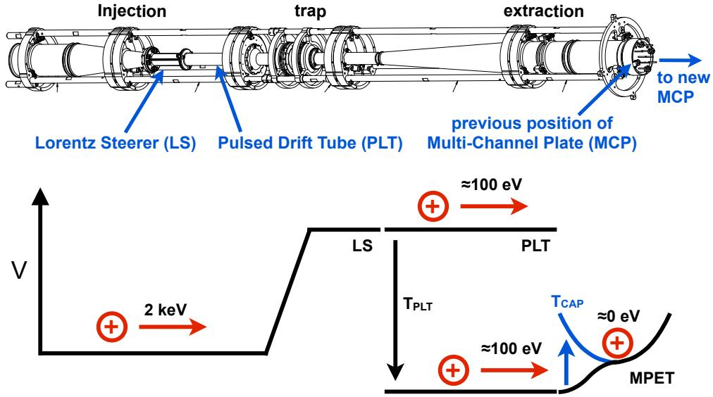
**Figure 3.32:** Top: Technical drawing of the injection, trap, and extraction setup of TITAN’s Measurement Penning Trap (MPET) structure. The whole structure is located inside a titanium vacuum tube placed in the bore of the superconducting magnet. The figure at the bottom explains the electrostatic potentials on axis (not to scale) and timings for the dynamic capture of ions in the MPET.
