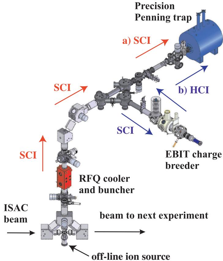
**Figure 3.2:** Schematic of the experimental setup of TRIUMF’s Ion Trap for Atomic and Nuclear science (TITAN). The different paths for SCI (a) and HCl (b) are marked.
