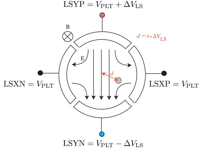
**Figure 3.34:** Cross sectional schematics of the Lorentz steerer. Figure modified from [146].
