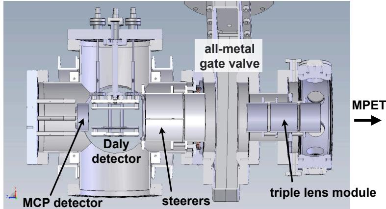
**Figure A.9:** Rendered technical drawing of the new optic elements on the extraction path to guide the ions to the new position of the MCP. A Daly detector is shown which has also been installed in the same 8” 6-way cross.
