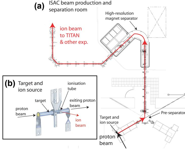
**Figure 3.3:** (a) Schematics of production, ionization, and separation of radioactive beams at ISAC. The inset (b) shows the target and ion source setup. Figure from [146].
