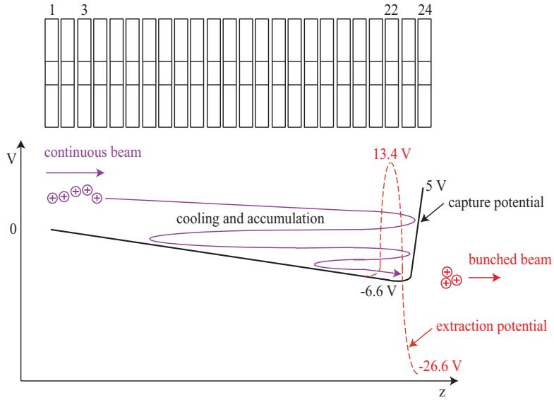
**Figure 3.8:** Top: Schematic of the longitudinal segmentation of TITAN’s RFQ into 24 sections. The segment number is indicated at the top. Bottom: Schematic of the typically applied potential. The DC field drags the buffer gas cooled ions to the minimum of the trapping potential (solid line). The beam is extracted in ion bunches by switching the potentials of the electrodes 22 and 24 (dashed-line). Figure from [146].
