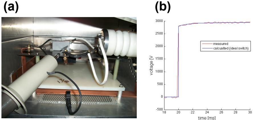
**Figure A.3:** Performance test of the PLT’s HV switch circuit with a high voltage probe (a). The measured signals are compared to calculations assuming an ideal switch in (b). The test has been done for switching from ground potential to 3 kV.
