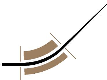
Figure 3.15: SIMION [44] simulation of a spherical bender. The bender not only steers the beam through forty five degrees but it also focuses the beam in both the bend (shown) and the non-bend directions.
