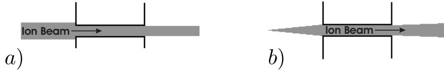
Figure A.1: (a) A wide parallel beam enters a narrow tube. A large proportion of the beam is lost. (b) A narrow diverging beam enters a narrow tube. Again a large proportion of the beam is lost.
