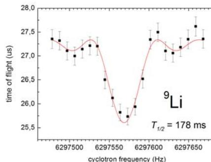
Time-of-flight resonances recorded by the TITAN Penning trap for (left) stable  $^6\text{Li}$  and (right)  $^9\text{Li}$ , produced from an ISAC Ta target in August 2007. The excitation times were 400 ms (left) and 20 ms (right). The lines are a fit of the data to the theoretically-predicted distribution [Koen1995]. Note that the sidebands, due to time-gated RF excitation, play an important role in reducing the uncertainty of the center frequency.
