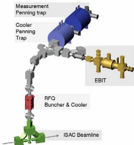
To make a mass measurement, an ion is injected into the homogeneous field of the TITAN Measurement Penning Trap (MPET) where its cyclotron frequency  $f_c = qB/2\pi m$  is probed and determined using a time-of-flight detection of the ejected ions. The cyclotron frequency is compared to that of a well-known reference mass (generally, a stable species of similar mass) to provide a measurement. TITAN was commissioned in August, 2007 at which point the masses of the short-lived
