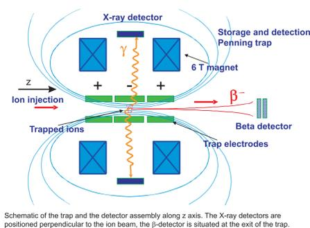
Schematic of the trap and the detector assembly along z axis. The X-ray detectors are positioned perpendicular to the ion beam, the  $\beta$ -detector is situated at the exit of the trap.
