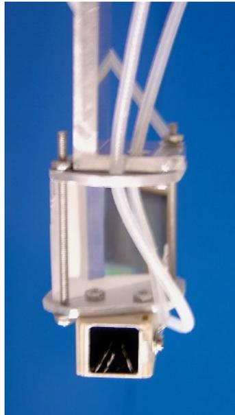
**Figure 3.31:** The channeltron and prism installed between the magnet and electron gun chambers. As shown, the entire assembly is mounted upside down. The channeltron horn faces the collector and is in the middle of the beam path, when the linear feedthrough it is mounted on is fully extended. The prism can be used to reflect light from the cathode towards the left, out through a vacuum viewport.
