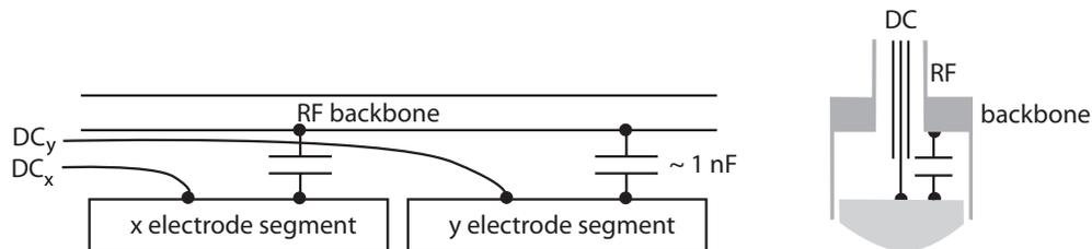
Fig. 5. A schematic of a scheme for superimposing a small DC potential on a large RF potential.
