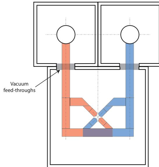
Fig. 8. A cross-section of a suggested configuration for an RFQ beam cooler driven by a half-wave resonator.
