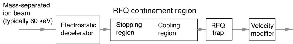
Fig. 2. A typical RFQ system for cooling and bunching an ion beam.
