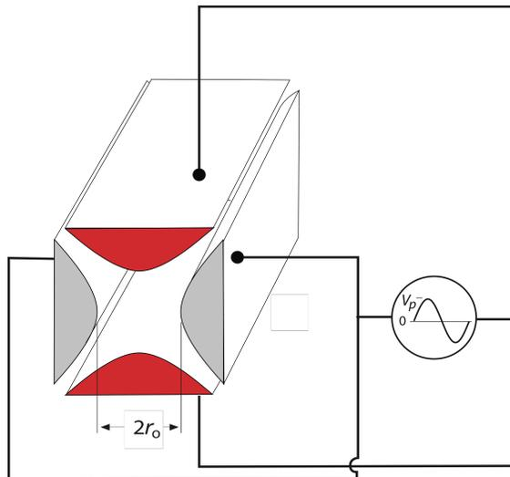
Fig. 1. A schematic of the RFQ structure and electrical potentials that provide the RFQ confinement for beam cooling and collecting.
