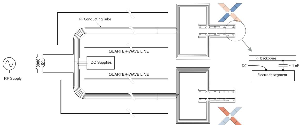
Fig. 6. A schematic of a scheme for driving an RFQ beam cooler based on a half-wave transmission line. Cross-sections of the RFQ electrode configurations showing the electrode pairs that are fed by the opposite ends of the half-wave transmission line are shown in the inserts.
