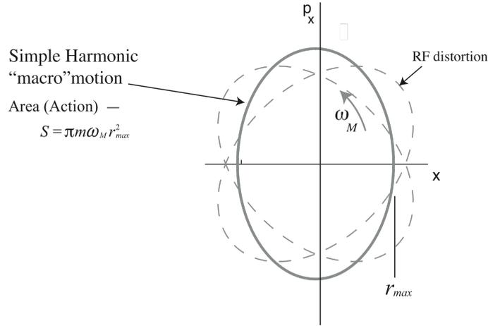
Fig. 4. The action diagram of particles under RFQ confinement. The action for the simple harmonic macromotion is shown as a solid-line right ellipse, the “x” semiaxis being simply the amplitude of the motion and the momentum semiaxis being this amplitude multiplied by the ion mass and the angular frequency of the macromotion. Representative cases of the distortion due to the driven RF motion are shown as dashed ellipses.
