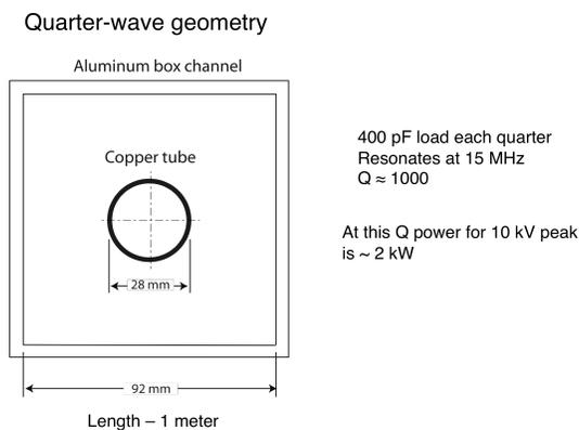
Fig. 7. A cross-section of one side of a mock-up half-wave transmission line for driving an RFQ beam cooler system. The length given is for each quarter wave.
