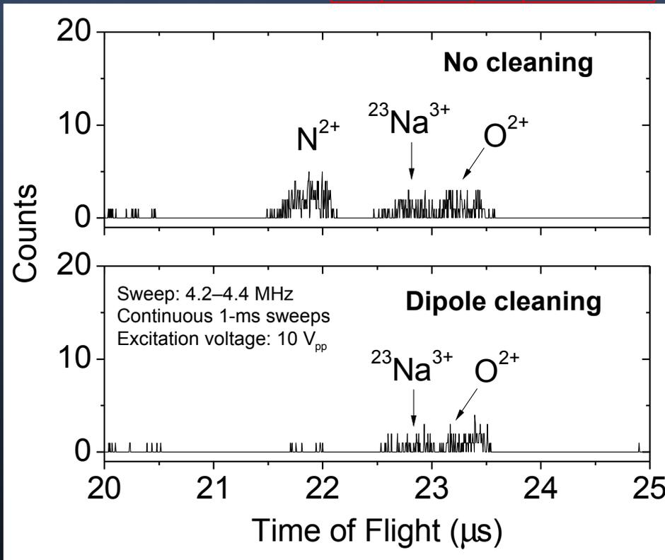
An RF dipole excitation sweep around the cyclotron frequency of  $N^{2+}$  removes this ionic species from trap.
