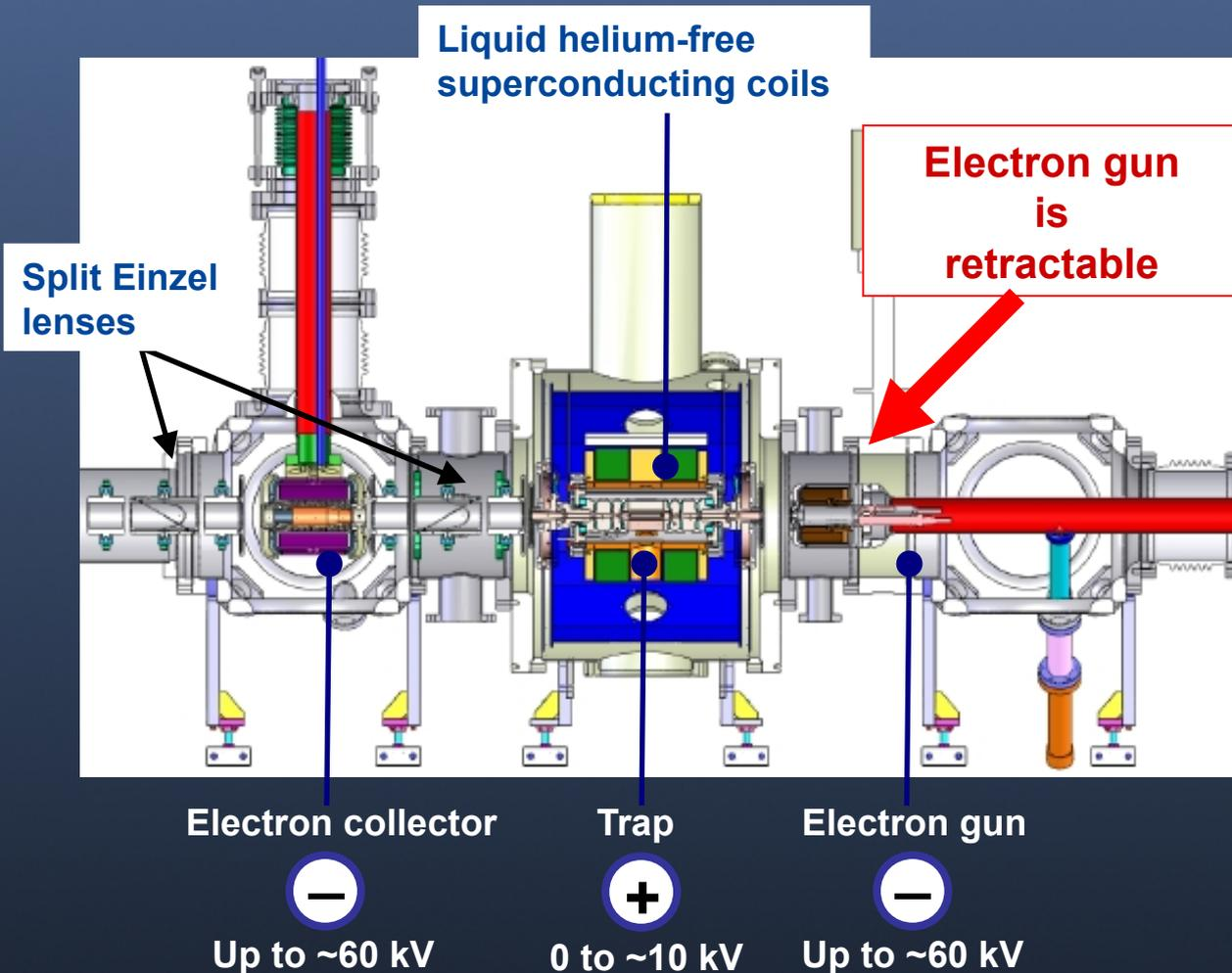
The gun & collector must be biased at high voltages to reach high electron beam energies.
