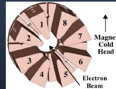
8-fold segmented central drift tube:
