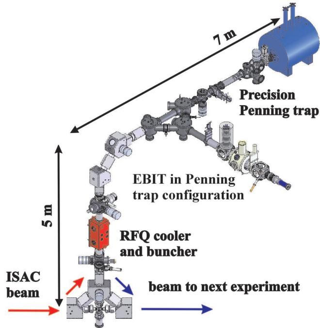
Figure 1: The TITAN mass spectrometer setup at the TRIUMF-ISAC radioactive beam facility. The EBIT is employed in Penning trap mode.
