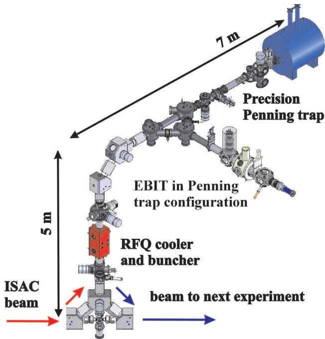
Figure 1: The TITAN mass spectrometer setup at the TRIUMF-ISAC radioactive beam facility. The EBIT is employed in Penning trap mode.
