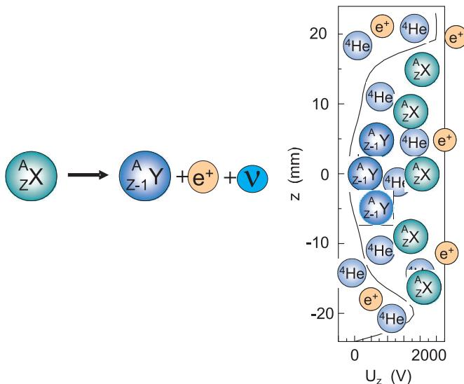
Figure 2: The beta-decay of an element. In the TITAN EBIT, employed in Penning trap mode, and filled with He-buffer gas, the recoil ions can be recaptured.
