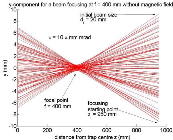
The final beam size is minimized according to three parameters before adding any optical elements:
