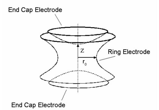
This electrode configuration can be used to trap ions with respect to the Z-axis and cause the ions to oscillate with a simple harmonic motion.
